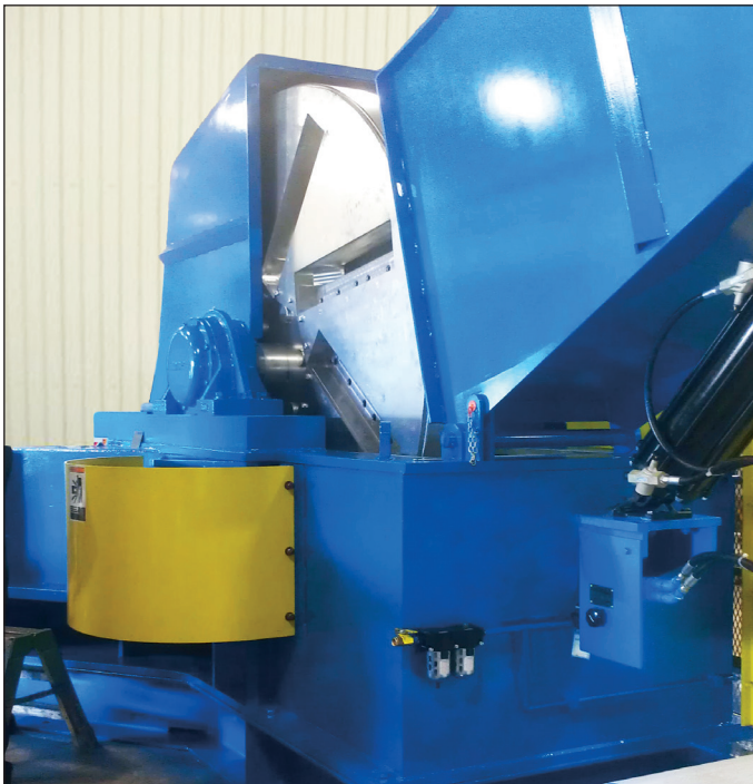
Cylinder-operated quadrant opening
