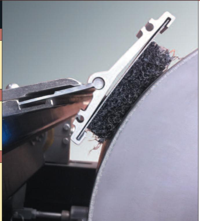
Doctor blades are used to remove contaminants and other matter from roll surfaces. Over time, the build-up on the roll surface requires additional cleaning to ensure more uniform roll surface conditions.
